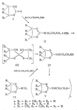
with an amine<sup>8</sup> have been reported. The reaction of 2-methylthio-4,4-dimethyl-2-oxazoline (VIa) and 2-mercaptoethylamine hydrochloride proceeded normally to 2-(2-mercaptoethylamino)-4,4-dimethyl-2-oxazoline (IVa), which could be isolated as the picrate. Treatment of the reaction product with base in the air yielded the disulfide Va.
